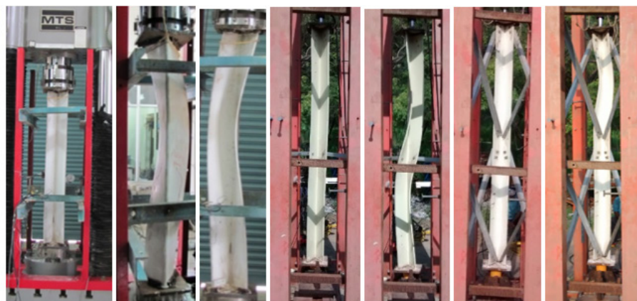
Fig. 3: Behaviour of 60^\circ angle section without and with intermediate redundant members
